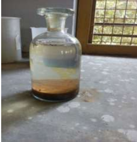
Fig. 4. Jar Test for Soil Texture
