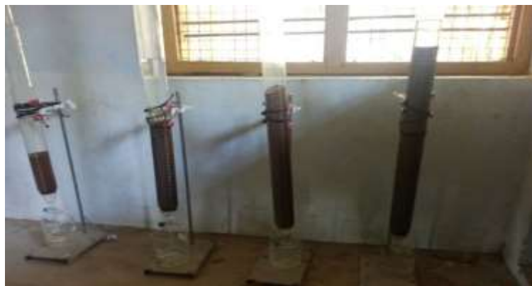
Fig. 3. Experimental setup for Column Study at Different Bed Depth
